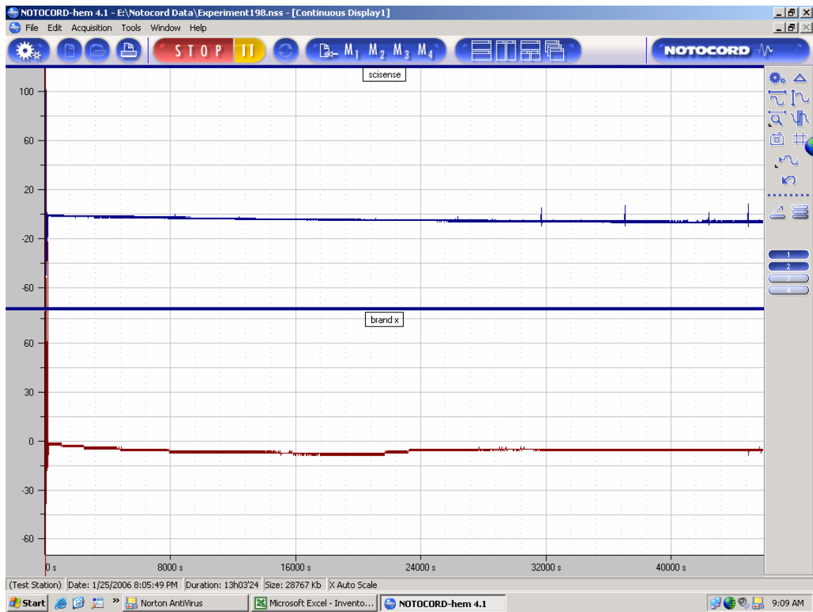
Figure 3: The plots show 12-hour drift rates of less than 5mmHg for both the Scisense and the Millar sensors.
